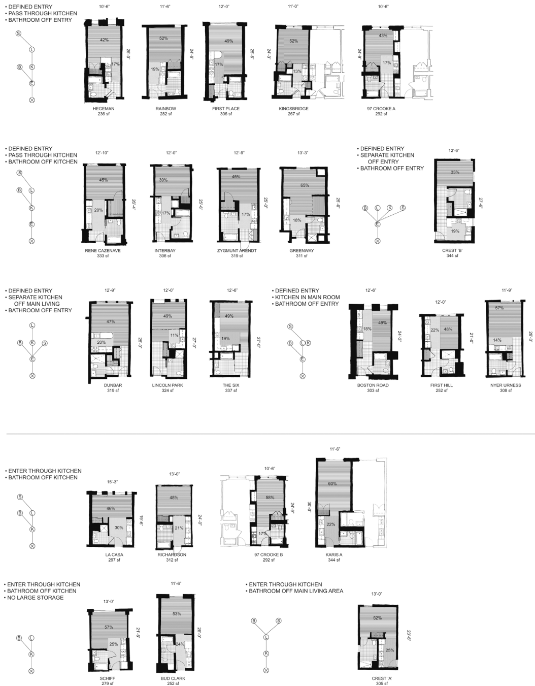
FIGURE 1 Sample units with floor area, dimension, and room organization arranged by typological category.
